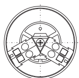
Single-phase capacitor with d = 60/70 mm Spring tension terminal AKD 25/2 for 2 \times 6 \text{ mm}^2
